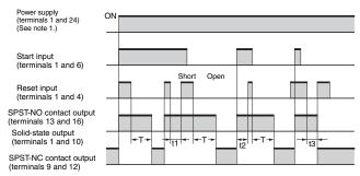
Note: 1. When using a 12/24 V DC-operated model with a 12 V DC power supply, short terminals 13 and 15.
