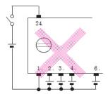
Input Terminals 2, 3, 4, and 6 Connected to the Negative Side of the Power Supply without Being Connected to Power Supply Terminal 1 (\*2)
